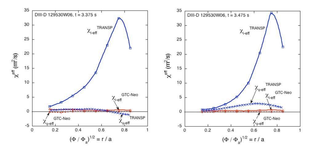
• For these two DIII-D cases, ion energy transport is strongly anomalous, as is also the angular momentum transport (though much smaller)
