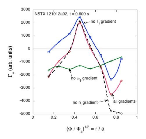
• Here  $\Gamma_{\phi}$ , the radial flux of toroidal angular momentum, is shown for an NSTX case (in internal code units) versus r/a (the square root of the normalized toroidal flux)
