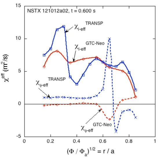
• Here we show  $\chi_{\phi}^{eff} = \Gamma_{\phi} / [R^2 n_i m_i (d\omega_{\phi}/dr)]$  (in m<sup>2</sup> / s) versus r/a for the same NSTX case, along with  $\chi_i^{eff} = Q_i / [n_i (dT_i/dr)]$ , both from GTC-Neo (neoclassical) and from TRANSP (experimental)
