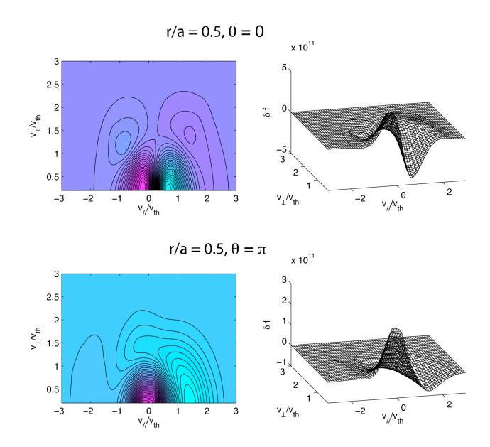
Contour plots and perspective plots of δf on outboard midplane and inboard midplane
